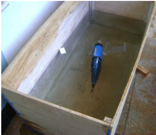
Fig. 6. Wooden box for testing the robot bump sensor. The robot is made to swim inside it in a tight circle
