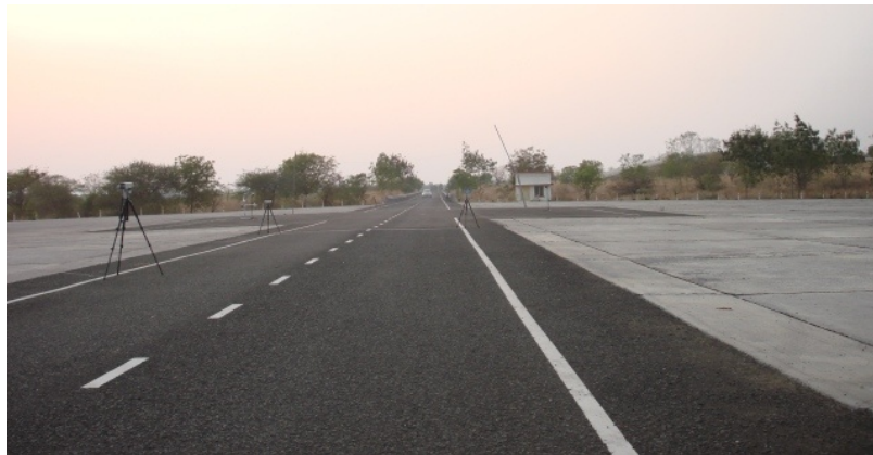
Figure 3: ISO 10844 test surface used for testing
