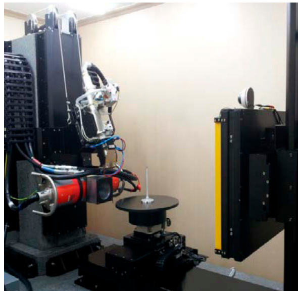
Figure 1. The CT(Computed Tomography) equipment with a high-power X-ray tube (450 kV/max, 1500 W).
