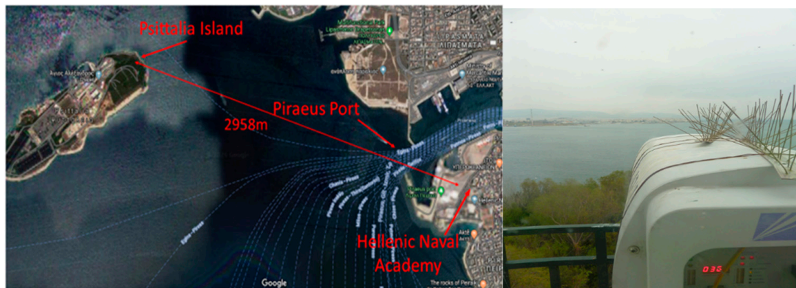
Figure 1. The maritime free-space optical (FSO) link propagation path (left) and the MRV TS5000/155 FSO terminal on the lighthouse of Psitalia Island (right). On the upper left back side of the system, the received signal strength indicator (RSSI) indicator can be seen.
