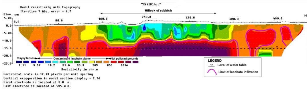
Fig. 9b. ERT SW-NE section showing the water table – leachate plume contact
