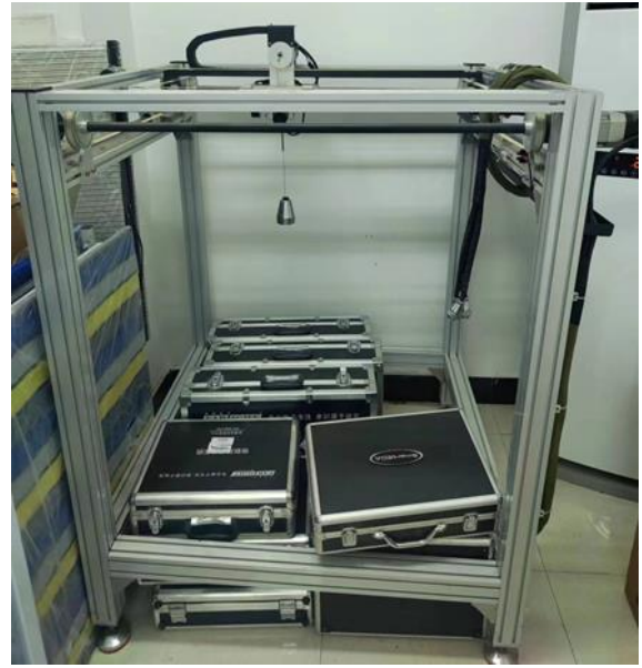
Fig. 1. Experimental equipment of the 3D bridge crane
