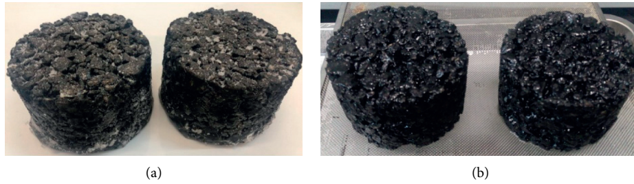
FIGURE 3: Process of freezing and thawing the test samples. Specimen appearance (a) after freezing and (b) after melting.
