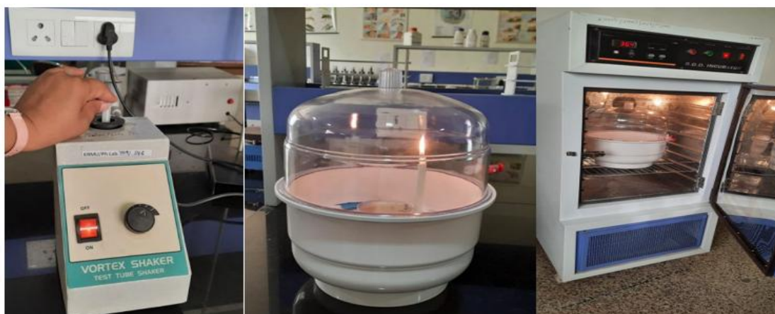
Fig. 1. A) Vortexing of the curd culture mixed with 0.9% sterile saline. B) Anaerobic environment provided to microorganisms by candle jar method. C) Incubation in BOD incubator at a temperature of 37°C
