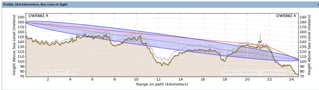
Fig. 3. Fresnel zone and Line of Sight (LoS) blocked by terrain profile
